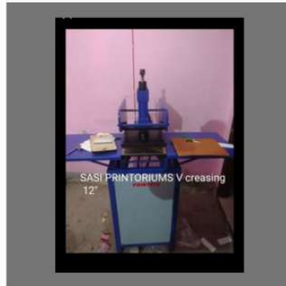
Dye 12 " Mini V Creasing For Paper Bottom Bags Handle D Cut , Handle Holes Foil Printing Machine
